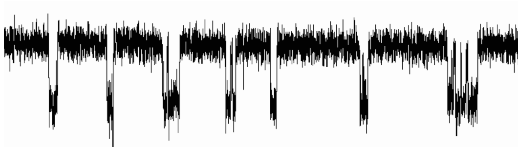
Figure 2.10: A typical single channel recording from patch clamp. The quantized currents occur due to two basic ion channel configurations: open and closed. Figure from Wikimedia Commons (2006).
